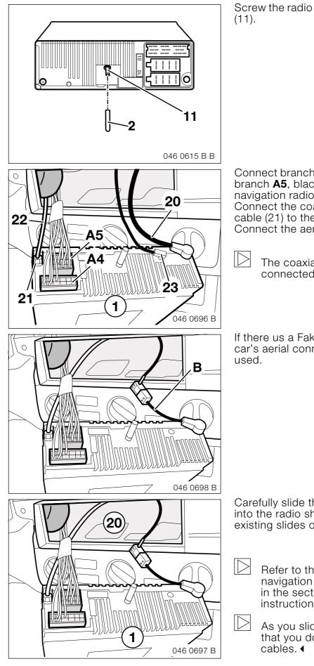
Screw the radio retaining pin (2) on to the stud bolt (11).
