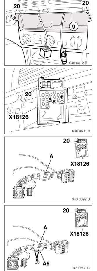
Insert the radio trim (9) and secure it with the existing Philips screws (20).
