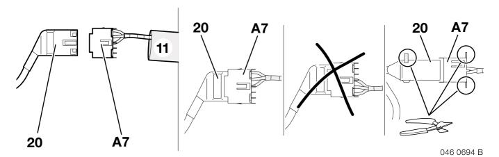
Push the shrink hose (11) over branch **A7**, silver 10-pin plug casing on adapter cable **A**, and connect the silver or black 10-pin socket casing (20) to the CD changer control cable.
