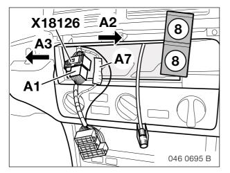
Connect branch **A1**, black 17-pin plug casing, to the 17-pin socket casing **X18126** on the audio wiring harness.
