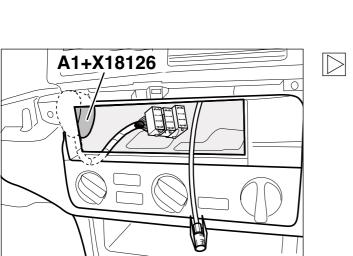
Lay the wrapped plug connector **A1+X18126** on the left behind the instrument panel so as to enable you to install the navigation radio.
