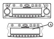
The volume is limited to a certain level after the display is folded down. After 20 seconds, a tone indicates that the control component is folded down. The unit then switches itself off.
